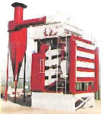
Maquinas de Limpeza de Cereais disponíveis nos modelos PL-130 (25 ton/h), PL-140 (35 ton/h), PL- 50 (40 ton/h), PL- 60 (60 ton/h), PL- 80 (80 ton/h).
